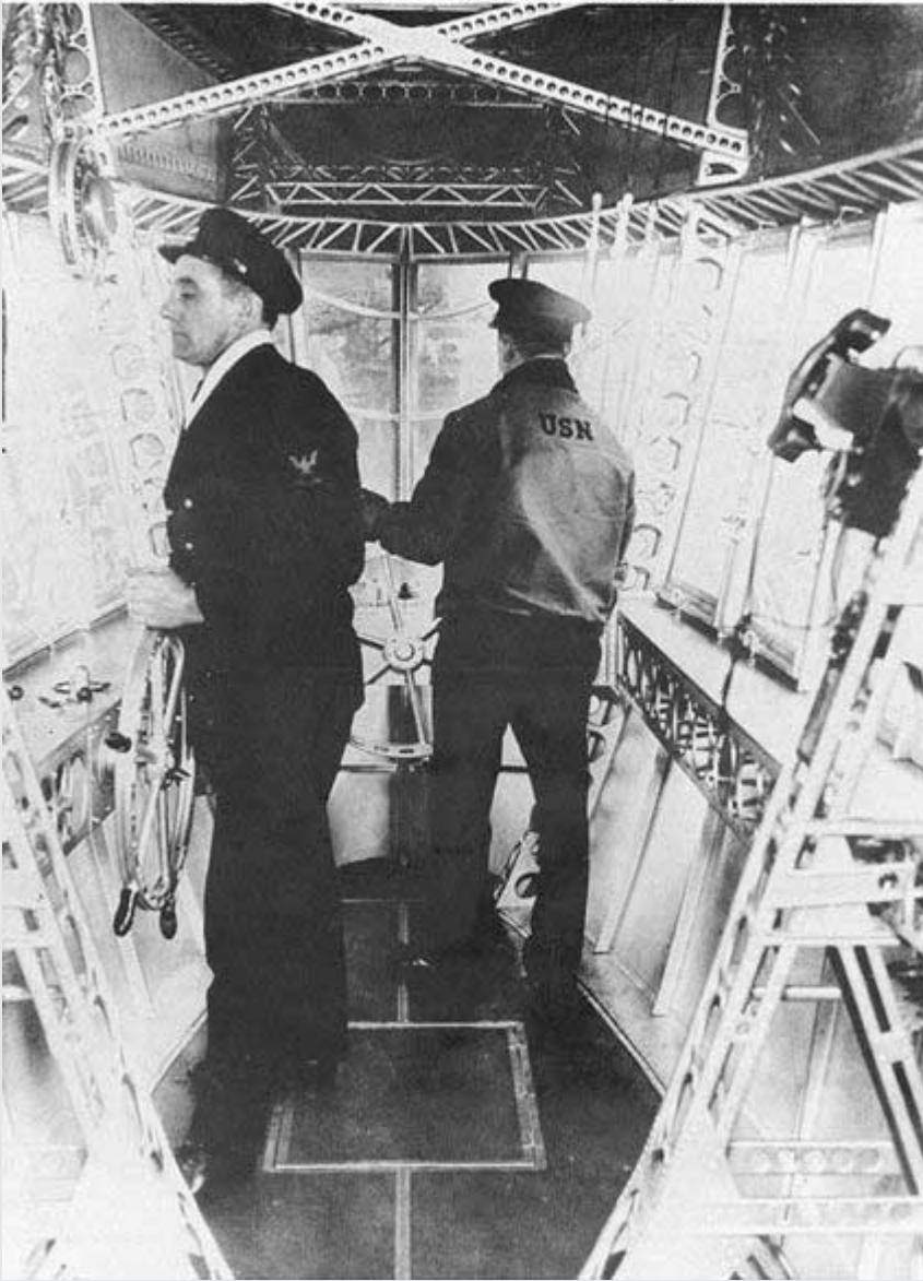
Photo # NH 82712 Interior of USS Macon's auxiliary control station
