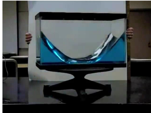
Fig. 1. Curvature of the water surface when the vessel rotates
